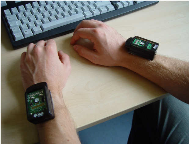
Figure 4.8: Positioning of sensor nodes with accelerometers, one per wrist.
