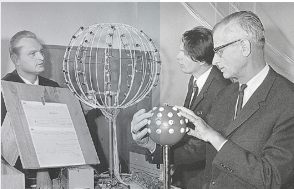
The spherical spatialisation controller for the World Expo 1970 in Osaka, developed at the Technische Universität Berlin, used by F. Winckel, M. Krause and C. Amberg in the background. | Photo Credit ► TU Archiv, 1970
