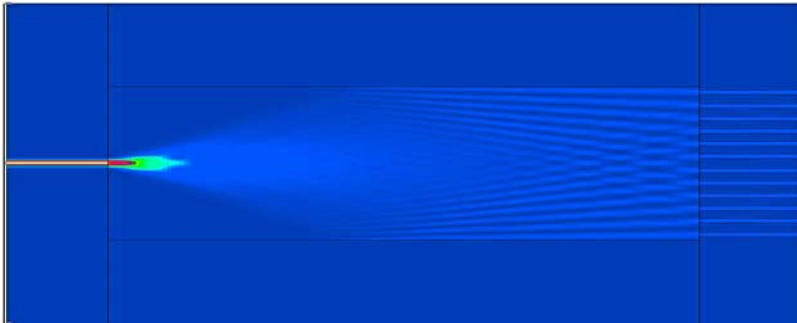
Figure 5.12: Simulation of the MMI coupler accommodating 12 laser ports, excitation from the left-hand side.
